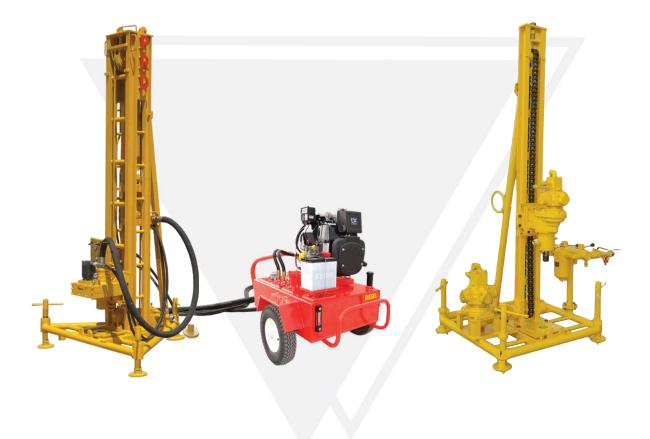
A portable bore hole drilling rig with a pull up force of 2700 kg capable of drilling 150 m of drilling 4" diameter up to 150 depth. Drilling hole size range from 4" - 6".
