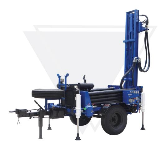
A compact bore hole drilling rig with a pull up force of 5100 kg capable of drilling 4  $\frac{1}{2}$ " diameters up to 150 m depth. Drilling hole size range from 4  $\frac{1}{2}$ " to 6".
