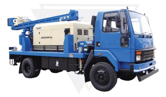
A highly compact bore hole drilling rig with a pull up force of 4450 kg capable of drilling  $\frac{1}{2}$  diameter up to 180 m depth. Drilling hole size range from 6  $\frac{1}{2}$  to 8".
