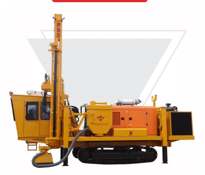
PRD 15 100 is a wise choice of blast hole rig for small scale mines with 100 – 165 mm diameter drilling. With 6000 kg pull down, 4 meter single pass depth and HVAC Cabin with all mining requirements fulfilled.
