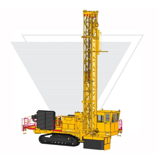
PRD 45 200 is a wise choice of blast hole rig for large scale mines with 165 – 240 mm diameter drilling. It is having 22000 kg pull down, 8.4 meter single pass depth and HVAC Cabin with all mining requirements fulfilled.
