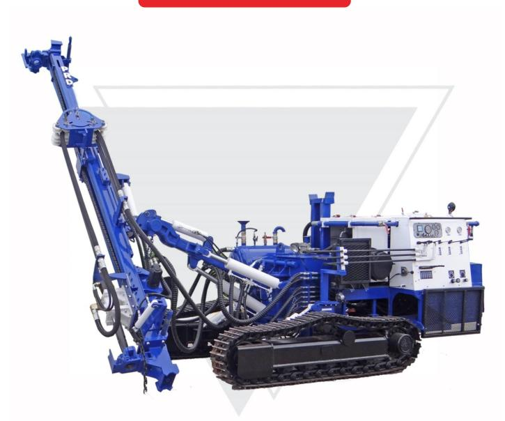
A perfect choice of small hydraulic rig for quarry drilling application with 1500 kgf pull down, Jack less rig with dust collector and water injection.
