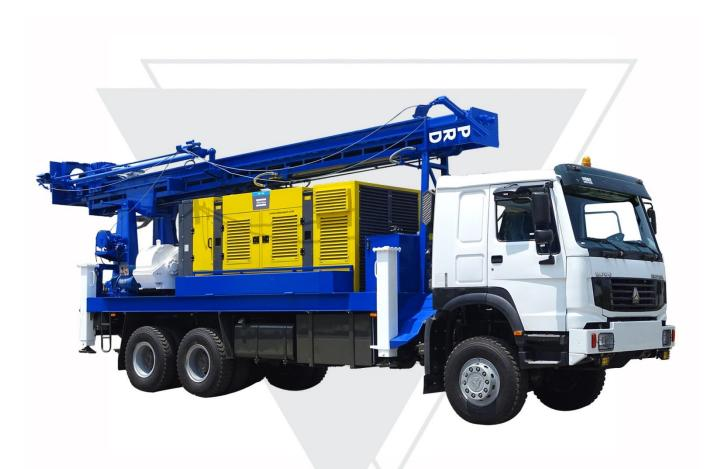
A combination bore hole drilling rig with a pull up force of 18000 kg capable of drilling 6  $\frac{1}{2}$ " diameters up to 600 m depth. Drilling hole size range from 6  $\frac{1}{2}$ " to 14".
