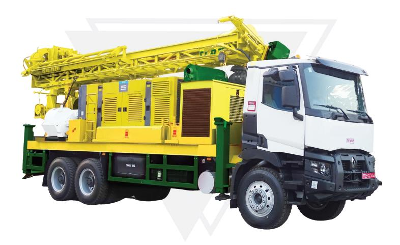
A versatile deep hole drilling rig with a pull up force of 25800 kg capable of drilling 6 ½" diameters up to 750 m depth. Drilling hole size range from 6 ½" to 20".
