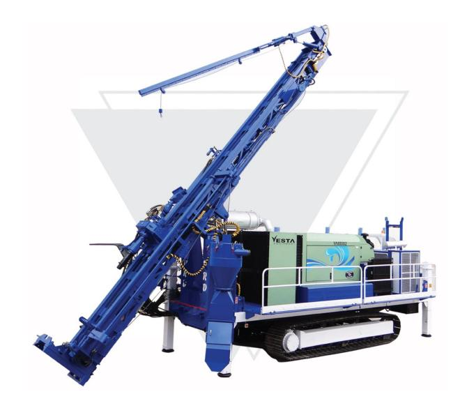
A robust & efficient sample recovery reverse circulation drilling rig with a pull up force of 25800 kg capable of drilling 5 ½" diameters up to 400 m depth.
