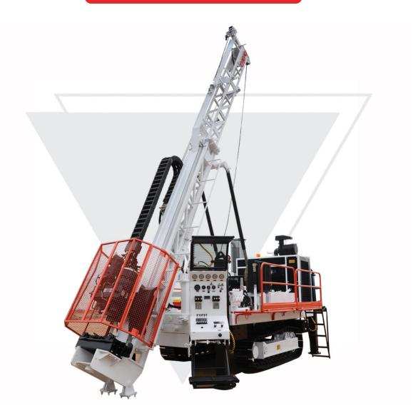
Miners preferred surface core drilling rig capable to drill 1250 m of NQ size. High speed chuck drive rotary head can do HQ, PQ, NQ & BQ drill sizes.
