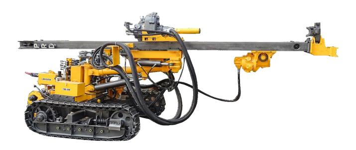
`PRD PC 500 crawler mounted pneumatic drilling rigs powered by air compressor. It is designed for aggregate quarry, limestone, construction and surface mining. The rig performs efficiently and compact, the power is fully utilized, low operating costs and top productivity.
